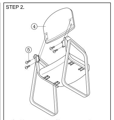
Align (4) backrest to (1) steel frames as shown. Then, screw-in with (5) backrest screws . Adjust (1) steel frames to reach the balance stand point . Securely tighten screws including screws of (3) seat.
